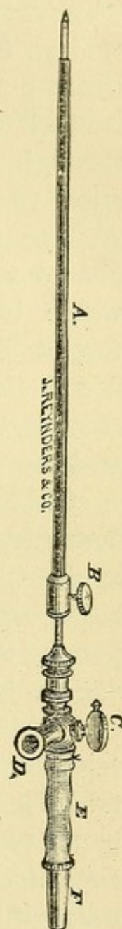
FIG. 37. GOELET'S TROCER AND CANULA.
