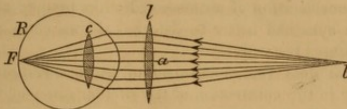
Fig. 60.— a b=6 inches. c =crystalline lens. R =retina. l =6-inch glass convex lens.
