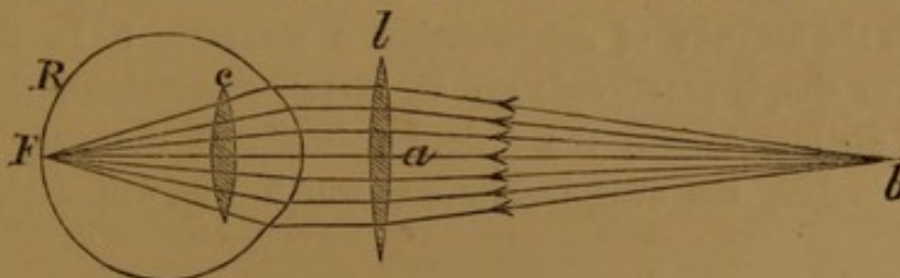
FIG. 57.— a b = 6 inches. c = crystalline lens. R = retina. l = 6-inch glass convex lens.
