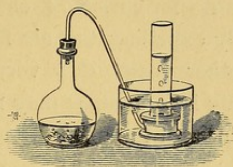
Fig. 19. Collecting the Gas evolved during Fermentation.
