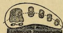
Transverse section of a well constructed Last, and proper sole.
