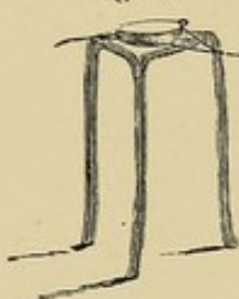
Wire triangles for supporting platinum capsules or foil while the organic matter is being burned off. p. 92
