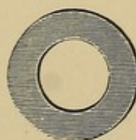
Ring used as an adapter for fitting various sized basins to the simple water bath. p. 92.
