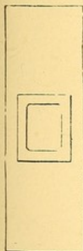
Simple glass cell for examining of urinary deposits. p. 97.
