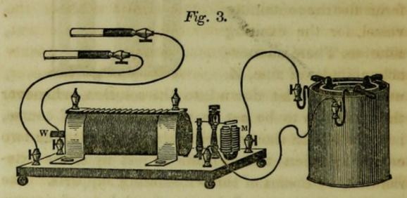
with the battery in Fig. 3. It consists, in its simplest form, of two concentric helices of wire, and in the axis of both, a rod of soft iron, or a number of iron wires. The current from the battery passes
