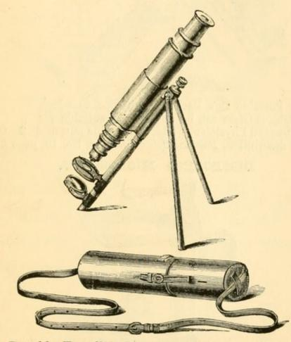
The Portable Travelling Microscope, a most useful Instrument for the Naturalist; to which any eyepiece, or object glass can be applied; it has quick and slow motion, and is supplied with Leather Case and Sling, into which it folds very compactly ... from 2 5 0 Vide description in *Microscopical Journal*, No. 26, page 20.
