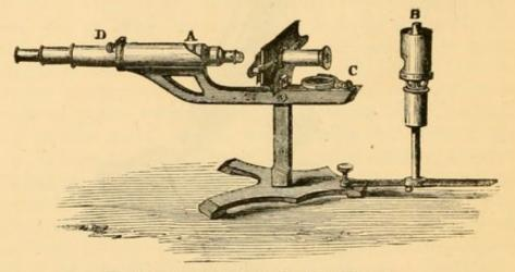
Fig. 58.-Murray and Heath's Class Microscope.
