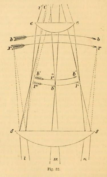
the field-glass, at the same time that it bends the rays and converges them to foci at b'b' and r'r', also reverses the curvature of the images as there shown, and gives them the form best adapted for distinct vision by the eye-glass *e e*. The field-glass has at the same time brought the blue and red images closer together, so that they are adapted to
