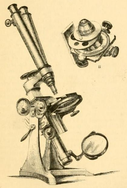
Fig. 39.—Ross's No. 1a Large Microscope, with Binocular arrangement and Object-glass. Scale 1/2.
