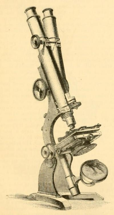
Fig. 47 .- Pillischer's No. 1 Binocular Microscope.
