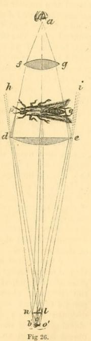
placed in any position; but the points of the image formed by a lens emitting no more than a small conical body of rays, which it receives from the glass, can be visible only to the eye situate within its range. Thus the pencil of rays emanating from the object at o', unless converged by the field-lens to f, would cross each other, and diverge
