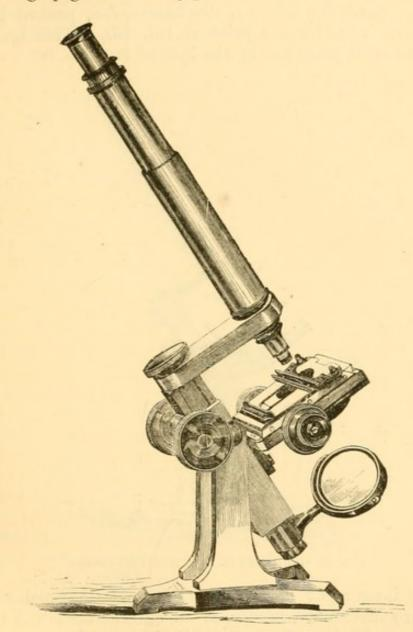
Fig. 48.—Pillischer's larger Student's Microscope.
