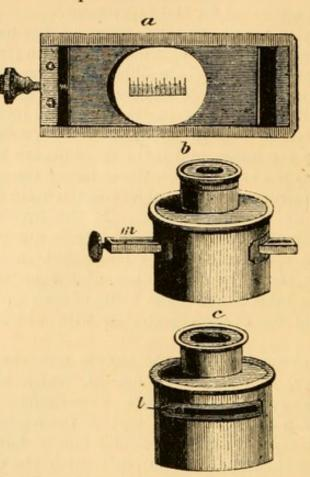
Fig. 35 .- Mr. Jackson's Micrometer eye-piece.
