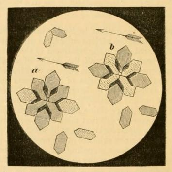
Fig. 92.—In this figure heraldic lines are adopted to denote colour. The dotted parts indicate *yellow*, the straight lines *red*, the horizontal lines *blue*, and the diagonal, or oblique lines, *green*. The arrows show the plane of the tourmaline, *a*, blue stage; *b*, red stage of selenite employed.
