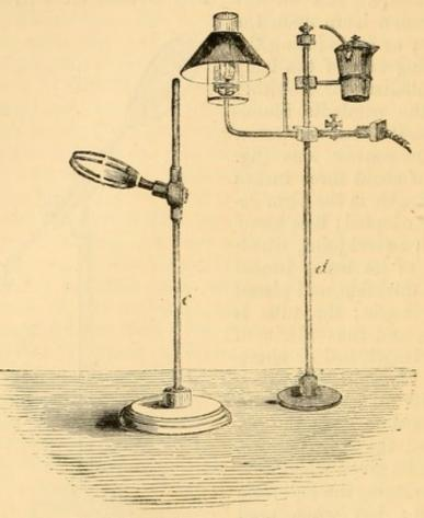
Fig. 107.-Condenser and Table Gas-lamp.
