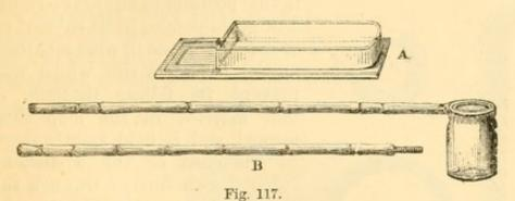
A. Trough for showing circulation in fish-tail. B. Collecting bottle and stick.
