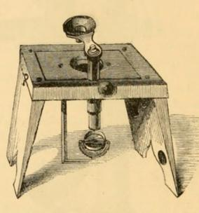
Fig. 25.-Quekett's Simple Microscope.
