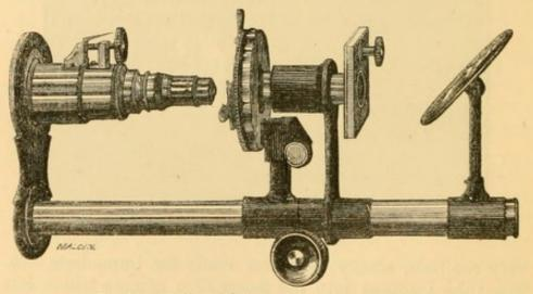
Fig. 97. - Highley's Photo-micrographic Arrangement.
