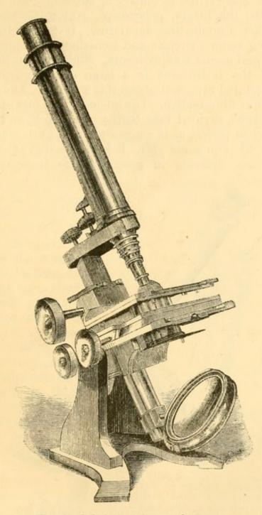
Fig. 43.—Baker's No. 2 Compound Microscope.
