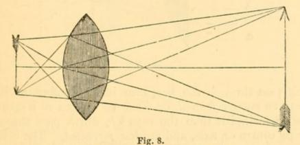
on the other hand, if the object be farther from the lens, the image will be nearer to it, and smaller than itself. But it is to be observed, that the larger the image is in proportion to the object, the less bright it will be, because the same amount of light has to be spread over a greater surface; whilst a smaller image will be much more brilliant.
