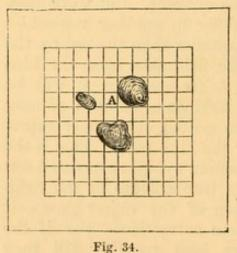
less. The markings of these divisions come into focus, therefore, at the same time as the image of the object, and both are distinctly seen together. The glass with its divisions is shown in fig. 34, on which, at A, are seen some magnified grains of starch. Thus the measure of the magnified image is given by mere inspection ; and the value of such measurements.
