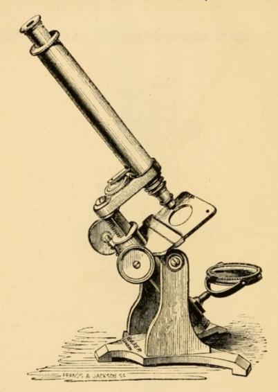
No. 4.—The Student's Microscope, a well-finished Instrument, with quick and slow motion, sliding object plate, a combination of three achromatic powers, live box, stage, and dissecting forceps, all packed in neat mahogany case ... ...
