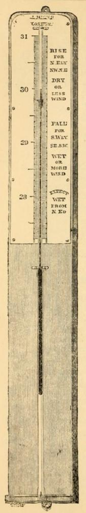
Hick's Open Range Barometer, giving from three to ten inches to an inch ... from 1 10 0
