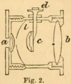
Between this knob and the inside and outside of the tube there are two slips of thin brass, which act as springs to keep the wire and disk steady. When the knob is moved, the injected object is carried to or from the lens, so as to be in its focus, and to be seen distinctly, whilst the condensing lens b serves to concentrate the light on the speculum. To the
