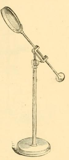
Fig. 106.-The Condensing Lens.
