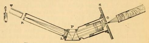
Fig. 69.-Sectional view of the Browning Spectroscope.
