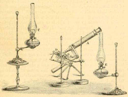
Fig. 103.-Mr. Newton Tomkins' Double Prism Illumination.
