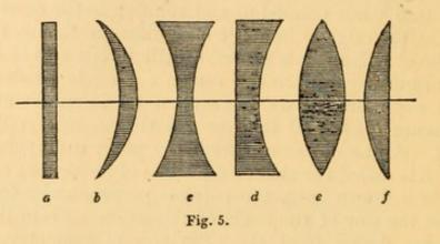
throughout; b, a meniscus, concave on one side, convex on the other; c, a double-concave; d, a plano-concave; e, a double-convex; f, a plano-convex.
