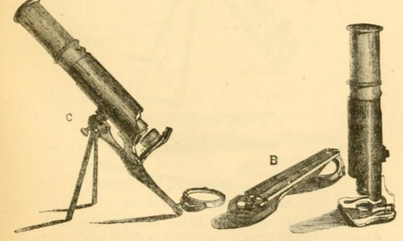
Fig. 62.-Murray and Heath's Sea-side Pocket Microscope.
