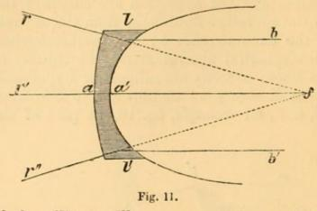
focus of the ellipse, will cause parallel rays b l, b' l', to diverge in directions l r, l' r'', which, when continued backwards, will meet exactly in the focus f, which will be its virtual focus.
