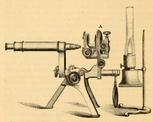
Fig. 36.—Powell and Lealand's Microscope arranged for Lobb's illumination. A. Secondary Stage carrying Achromatic Condenser.
