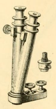
The Improved Binocular Arrangement, which allows the removal of the prism with its necessary fittings, so that when the monocular body is used, an uninterrupted field is obtained. Applied to any of the preceding microscopes ... from 5 0 0 To Student's or smaller instruments ... from 3 10 0 THE STUDENT'S MICROSCOPE, COMPLETE.
