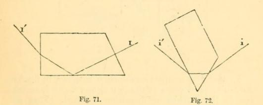
Figs. 71 and 72 represent prisms of the kind made by. Mr. Browning, used in two different positions, i and i' being the same angle as I and I'.
