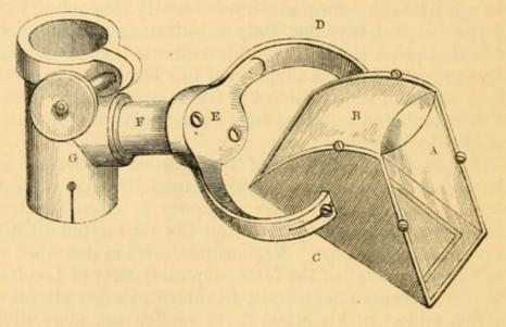
Fig. 101.—Abraham's Achromatic Lenticular Prism. Half-size.
