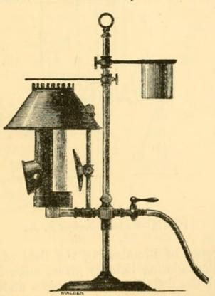
Fig. 109.-Highley's Gas-lamp, with Steam-bath attached.
