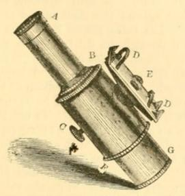
Fig. 75.—The Sorby-Browning Micro-spectroscope.
