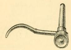
The New Finder, a simple piece of apparatus for registering the position of a diatom or any other minute object on a slide; attached to any microscope ... ... ... 0 4 0
