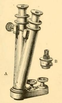
Fig. 45.-Baker's arrangement of Wenham's Binocular.
