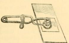
heat should be applied to drive Fig. 138, half size. -Spring-clip, showing its mode of application.
