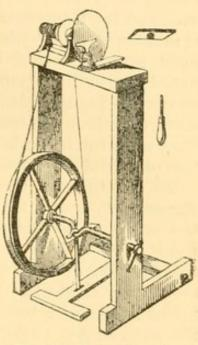
Fig. 135 — Small Lathe for polishing.
