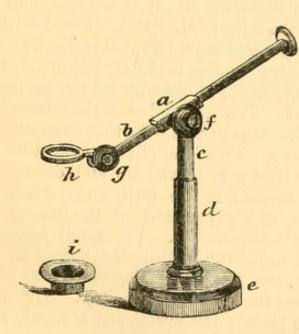
Fig. 23.-Ross's Simple Microscope.
