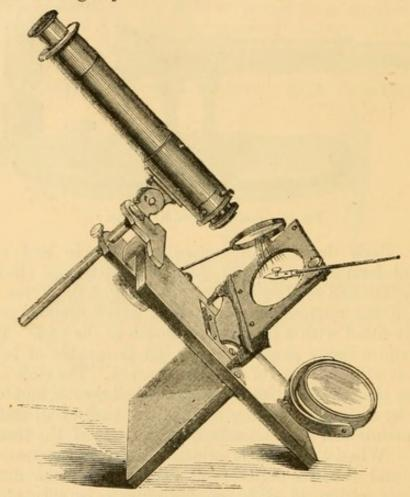
Fig. 60.- Warington's Universal Microscope.
