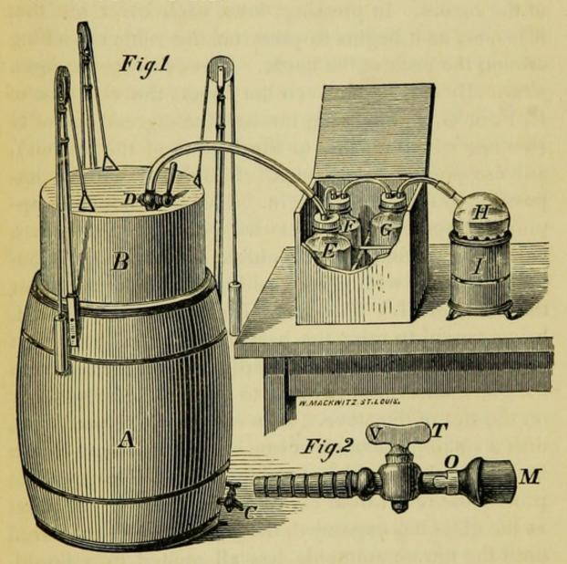
Arrange the apparatus as shown in the above diagram, Fig. 1. Observe, in unpacking, that the barrel A, (which forms a tank,) should be opened at the end marked O. Having removed the contents, place the zinc reservoir B, mouth down in A. Insert faucet C, (used in emptying the tank) in place. Screw on the
