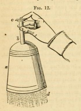
the bath, which is filled with water. The thumb of an attendant is then to be placed upon the orifice in the centre of the rim, (c) and the bath raised from the bucket of water. The pressure of the air upon the holes in the bottom retains the water in the bath, and on raising the thumb from the upper orifice, the water is rapidly discharged." (Fig. 12.) Portable shower-baths, holding from a quart to a gallon or more of water, are now made so that the patient may hold the vessel himself above his
