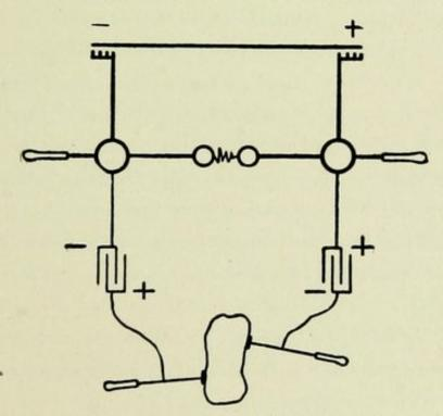
Fig. 4. Arrangement for the Static Induced Current.
