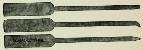
Fig. 12. Glass Sleeves for Use with Brush-Discharge.
