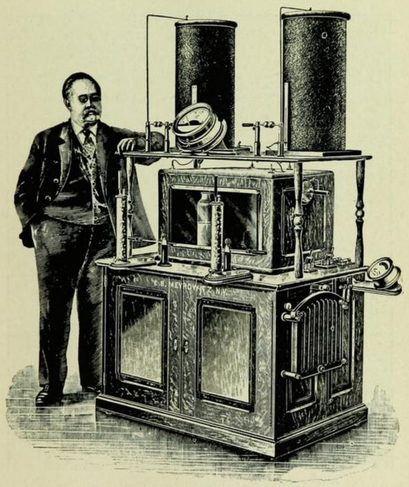
Fig. 17. Meyrowitz Coil and High-frequency Apparatus.
