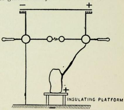
Fig. 1. Arrangement for the Static Wave-Current.
