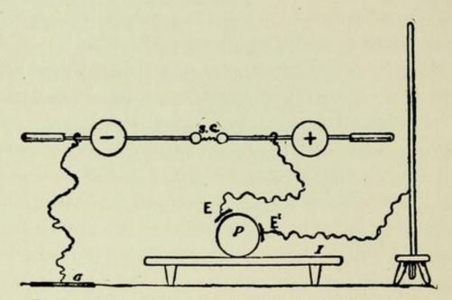
Fig. 2. Showing Arrangement with an Insulated Capacity.
