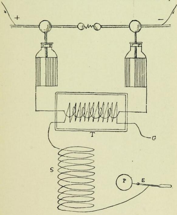
Fig. 6. Arrangement of Common Resonator.
