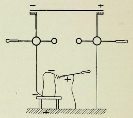
Fig. 5. Arrangement for Indirect Spark.
