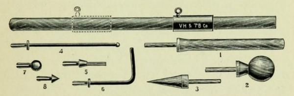
Fig. 11. Author's Set of Brush-Discharge Electrodes.
