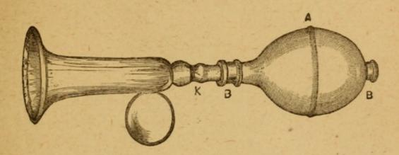
Desiring its removal, INSTANT RELEASE can be had by simply raising the Bulb, which opens vent "K" in the rubber tube connecting Bulb with the vacuum glass.
