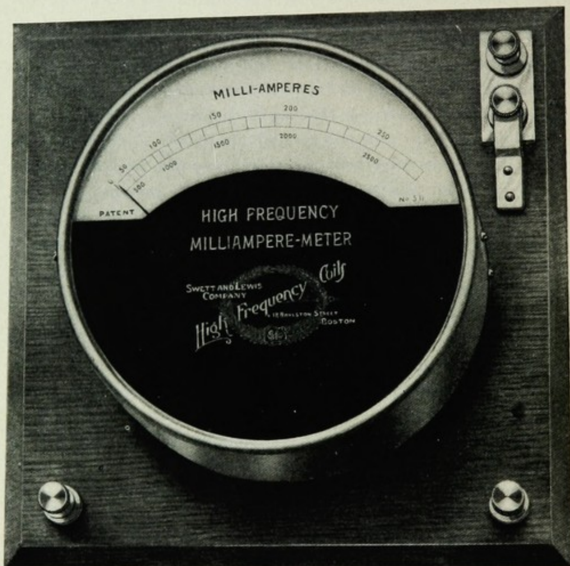
FIG. 104.—Hot Wire Milliampere Meter for Measuring the Intensity or Volume of Currents of High-frequency.
