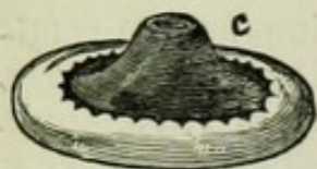
Carbon disk electrode covered with wash-leather.
