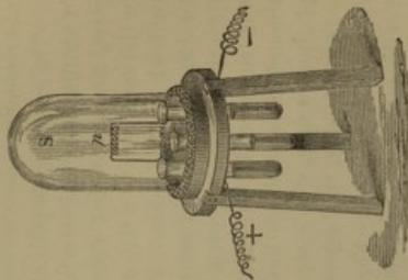
this sufficed for the entire removal of the floating matter. When the spiral was heated, a portion of the expanded air was driven through the cotton-wool packing below; and when the current was interrupted, this air, returning into the shade, was prevented by the cotton-wool from carrying any floating matter with it.
