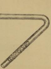
as in fig. 13, the inclined portion being plugged, so that no impurity could fall into the liquid from the cotton-wool. These two bulbs were boiled for five minutes in an oil-bath, and plugged while boiling with cotton-wool. They were then sealed behind the plugs and permitted to cool, their sealed ends being broken off afterwards.
