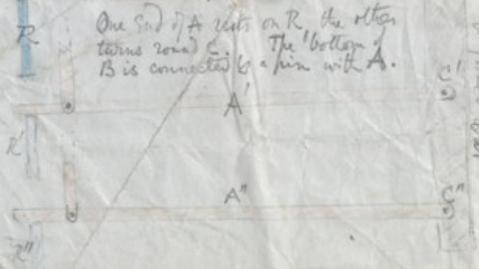
One end of A rests on R, the other turns round E. The bottom of B is connected by a pin with A.
