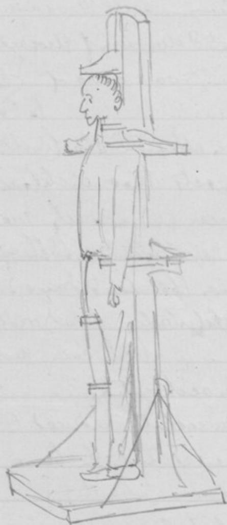
improved form was used. It enables a man to be measured & gauged all over. The various readings are taken after he has left the machine. — There are 3 views of this machine in p. 234.
