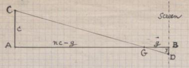
AB = distance of Camera from screen, measured along the horizontal ball AC = height of Camera .
