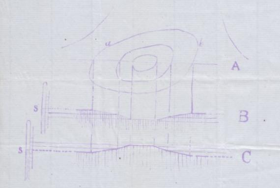
Isobaric plan of an area either of low or of high pressure.
