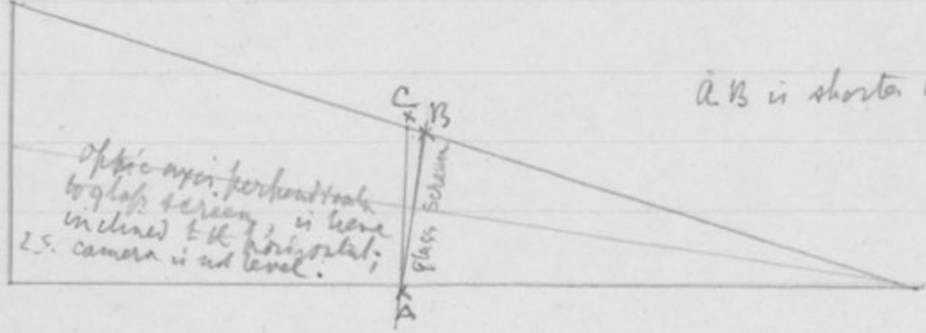
Optic axis perpendicular to glass screen, is here inclined to the horizontal; i.e. camera is not level.
