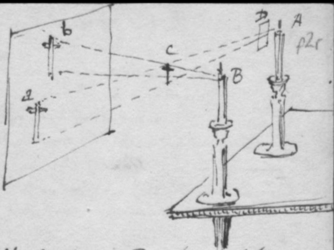
1/ Let A and B represent two candles, C an opaque object, held up in such a way as to receive the light of each of them, & thereby cast two shadows, (~~upon~~ a the shadows from A, and b from B,) upon a white sheet of paper or linen.
