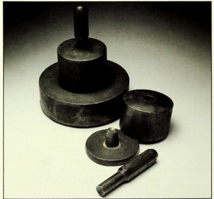
Right: Brockedon's original apparatus for the manufacture of compressed drugs, 1843
