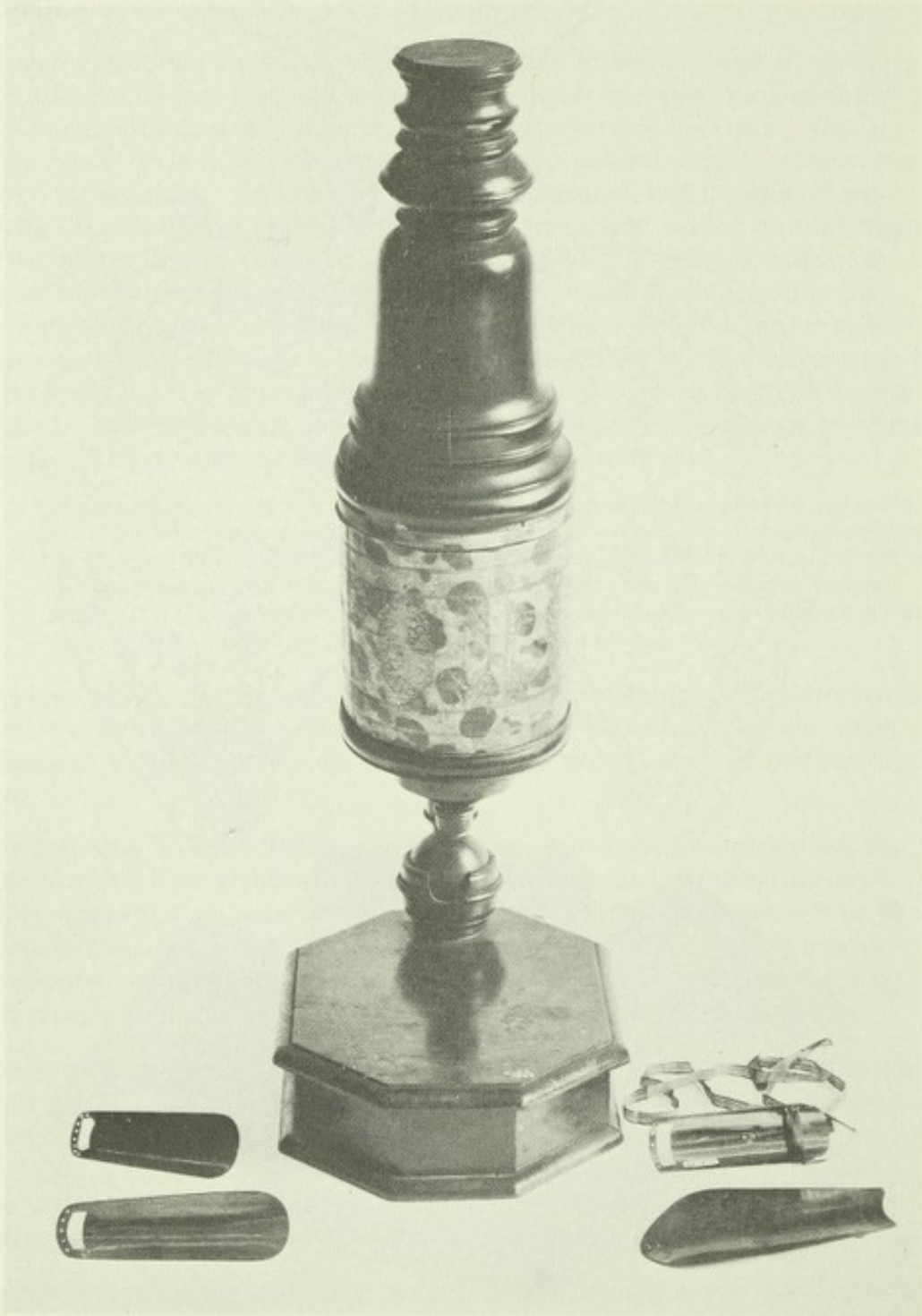
Illust. 9. 18th century Marshall microscope and brass holders for examining circulation in fish tails.
