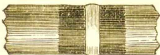
Fig. 32.—UNDERHAND JOINT, TOO SHORT AND TOO LIGHT.
