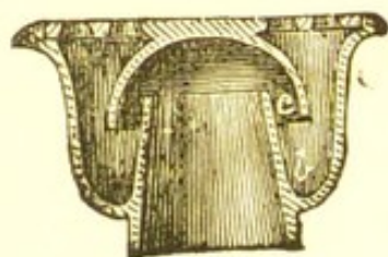
Fig. 78.—SECTION OF A BELL-TRAP.
