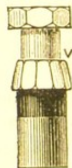
Fig. 59.—OVERCAST COPPER-BIT JOINT.
