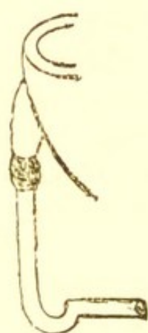
Fig. 135.— OVERFLOW- TRAP, IN- EFFICIENT SEAL.
