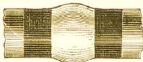
Fig. 38.—VIEW OF AN UNDERHAND JOINT.
