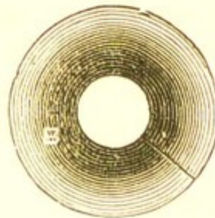
Fig. 40.—PLAN OF A LEAD COLLAR WHEN TURNED UP.
