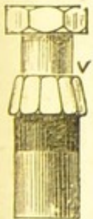
Fig. 18. Over-cast Copper-bit joint.
