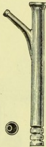
Fig. 119.—Kronecker's Perfusion Cannula, for supplying Fluids to the interior of the Frog's Heart.
