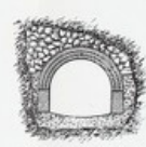
Fig. 168.—Tunnel at Clay or Soft Slips.
