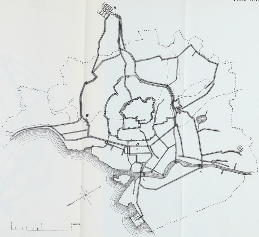
FIG. 184.—WATERWORKS OF TOKYO: DISTRIBUTION SYSTEM.
