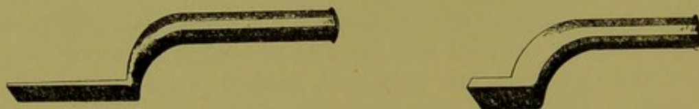
Figs. 203, 204.—Tools used for caulking joints of pipes.
