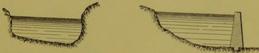
Fig. 16.—Diagram illustrating mean depth of reservoir with steep sides.
