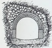
Fig. 168.—Tunnel at Clay or Soft Slips.
