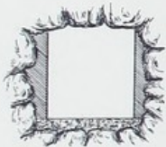
Fig. 167.—Tunnel at Decomposed Granite.
