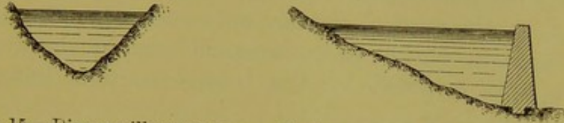
Fig. 15.—Diagram illustrating mean depth of reservoir with sloping side.
