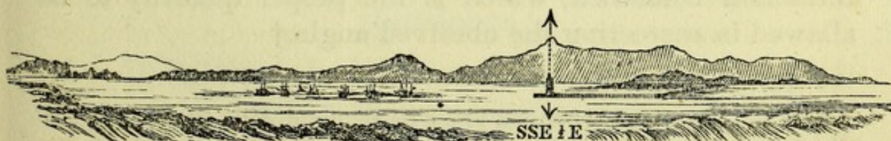
Lighthouse in one with East Peak of Mount Auckland, clears reefs in 4 fathoms, and kept open (S. by E.), leads through the passage, mid channel.
