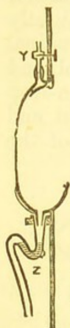
Fig. 239. We come now to urinals; but after what has been said upon wash-hand basins and sinks, I need not take up much space with them. They are of various styles—high-backed and low-backed, round-backed, flat-backed and cornered. Fig. 239 is section of a high-backed cradle urinal with a \frac{1}{2} -in. screw-down stop-cock at y, and a 2-in. lead syphon-trap at z. I have often used Lambert's \frac{1}{2} -in. stop-cocks for these urinals, the upper part of the round disc with the four screws in it being so exposed and finished flush with the wood as that the top cover could be easily unscrewed and a new india-rubber washer put in without removing any part of the wood lining. In addition to the foregoing exposed crane, another crane is often put on underneath the woodwork, somewhere
