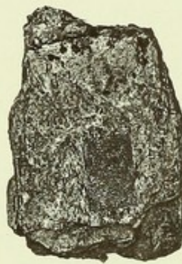
Piece of an Iron Plate converted by chemical action into a substance resembling decayed wood.
