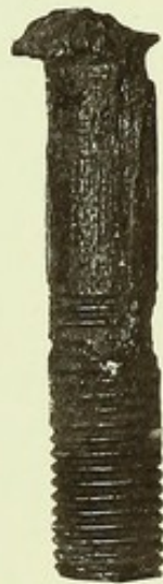
Bolt as taken from the Ship two years after.
