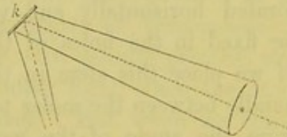
Fig. 4. k , Laryngeal mirror; to the right is the illuminating mirror, perforated. The continuous lines represent the outline of the luminous fasciculi which are interrupted at the laryngeal mirror k . The dotted line represents the visual axis of the eye placed before the mirror.
