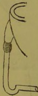
FIG. 142.—Overflow-arm badly trapped.
