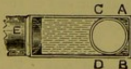
FIG. 18.—Plan of the "Narrow-band" D-trap.
