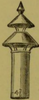
FIG. 262. — View of “Double - cap” Ventila- tor.
