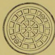
FIG. 207.—"Cobweb" Grating and Rim.
