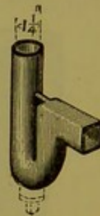
FIG. 31.—View of 1¼-in. "Anti-D-trap."
