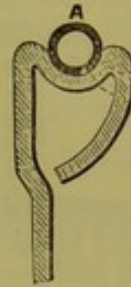
FIG. 148.—Section of Basin-rim with india-rubber packing, A.
