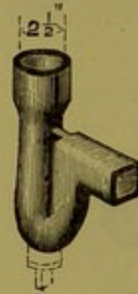
FIG. 30.—View of 1¼-in. "Anti-D-trap," with enlarged mouth.
