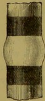
FIG. 131.—View of a Wiped Soldered Joint.
