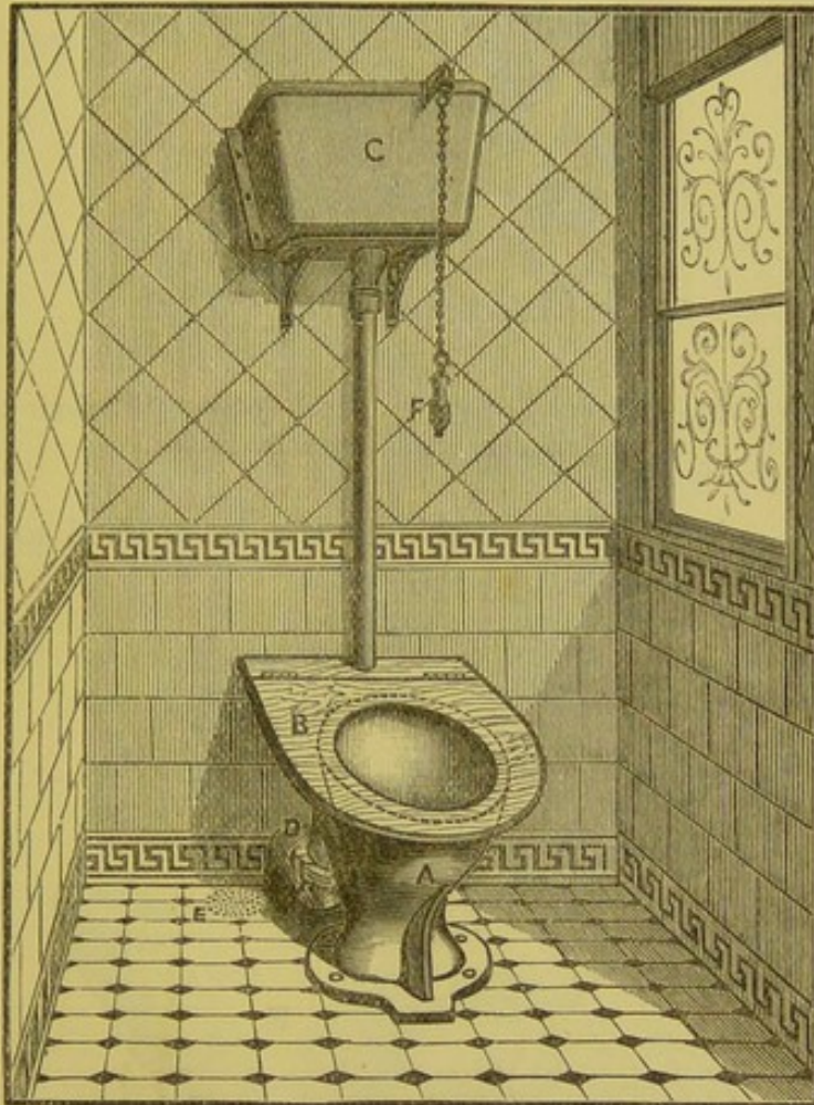
FIG. 272. —View of the "Pedestal" or "Hygienic" Closet, with a Syphon Flushing-cistern over it.
