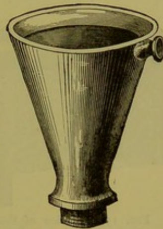
FIG. 154.—View of a Hopper-closet—bad shape.
