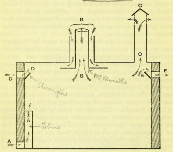
Fig. 1.—Ventilators. A A, Tobin's; BB, McKinnell's; DD, Sheringham's (acting as inlet); EE, Sheringham's (acting as outlet); CC, Ventilating shaft.
