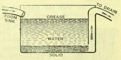
Fig. 14.-Grease Trap.
