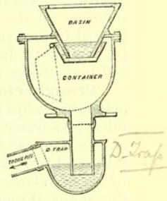
Fig. 20.—Pan Closet, with D-trap.
