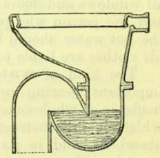
Fig. 19. — Wash-down or Short Hopper Closet.
