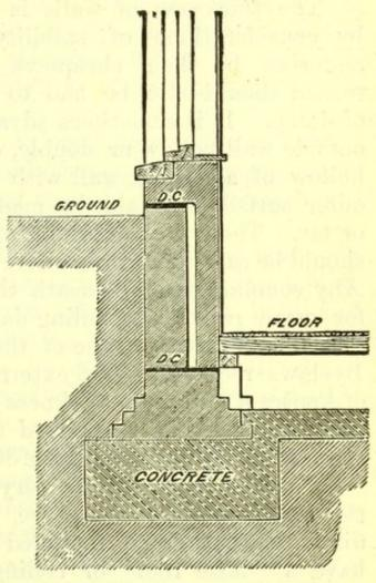
Fig. 7.—Double damp-course. Soil abutting upon hollow wall.
