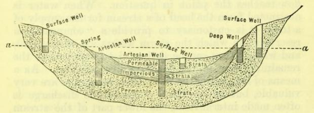
Fig. 5.—Diagrammatic Section across a Valley. a a, Level of water in deeper permeable strata.
