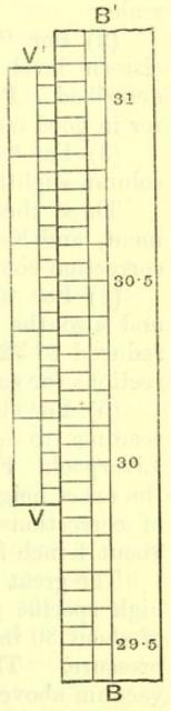
Fig. 2.—Barometer Scale and Vernier, showing a reading of 29.85 + 18 × .002 = 29.886 inches.
