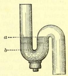
Fig. 8.—Siphon Trap (Strap) with access screwplug for cleansing. a, b, the seal.
