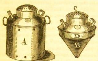
Steam and Spirit Lamp Bath. A, 6½ diameter, 8 deep to first rim. D, 1¾, B, 4½ deep; this sloping part holds a quart of water. C, perforated top. Inside A is a movable can, 3½ diameter, 2¼ deep, to hold a quarter pint of methylated spirits of wine, or rectified naptha, to place inside A; light the spirits, then put in can, C D, with sloping point B into the spirits. The
