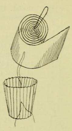
the milk to be tested, run on to the upper part from a pipette. The milk is rapidly absorbed by the paper and none filters through the cap. It is then dried in a water oven for an hour or two.
