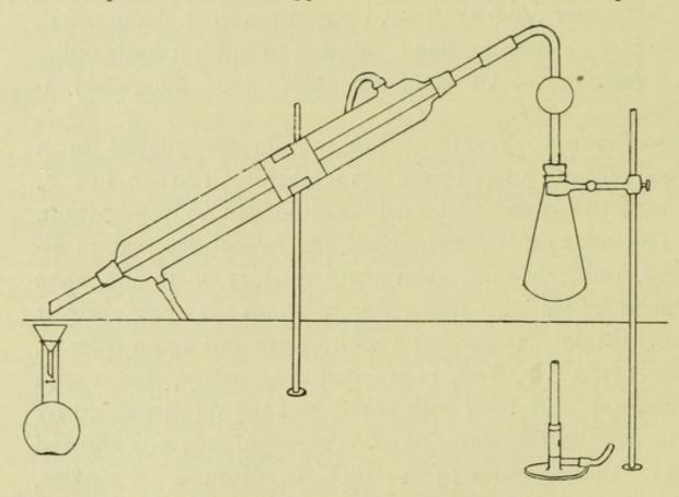
tions of water should be added drop by drop, and the flask shaken between each addition, in order to avoid foaming. When the soap is dissolved, 5 c. c. of the dilute sulfuric acid are added, a piece of pumice dropped in and the liquid distilled until 110 c. c. have been collected. The condensing tube should be of glass,
