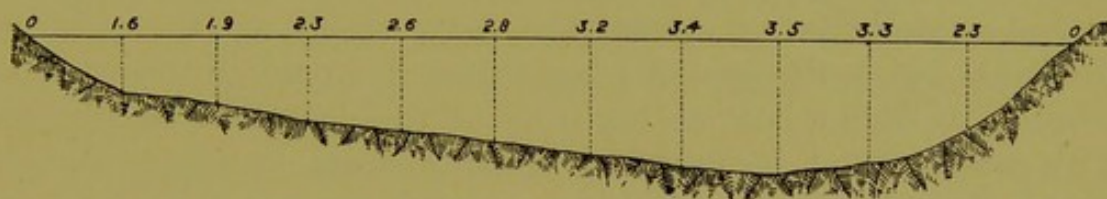
Fig. 4.—Section across river showing depth of stream at various points.
