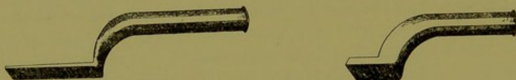
Figs. 203, 204.—Tools used for caulking joints of pipes.
