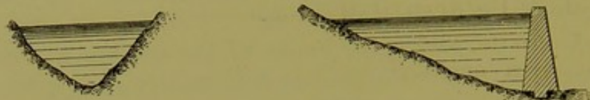
Fig. 15.—Diagram illustrating mean depth of reservoir with sloping side.
