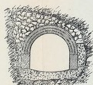
Fig. 168.—Tunnel at Clay or Soft Slips.
