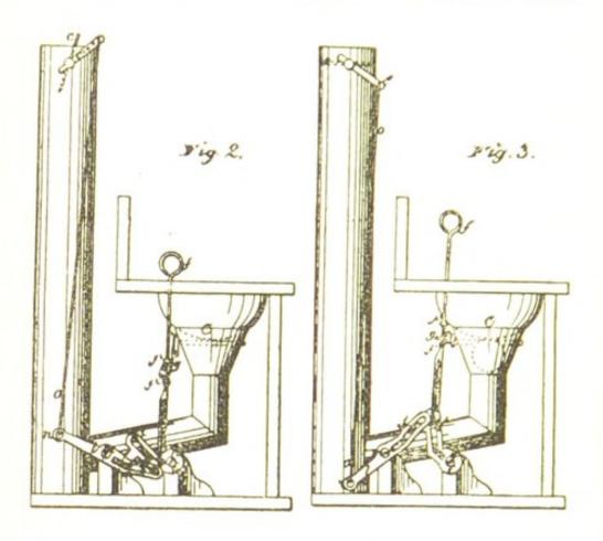
damper stands open. When the handle of the water-closet is raised, its first effect is to close the damper, and thus prevent the supplying of air from the summit of the soil-pipe; its further movement tilts the sealing-pan, and discharges the contents of the closet into the soil-pipe. As soon as the sealing-pan is open, the de-
