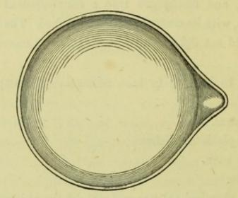
If there be many milks to examine, it will be well to have a set of the little dishes (which cost 14s. a piece, and which are numbered on the lip.) The dishes are to be cleaned and weighed, and the weights noted down: they will alter in weight only very slowly, and even if in active use, require reweighing only every now and then.
