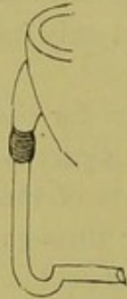
FIG. 155.— Showing overflow- arm badly trapped.
