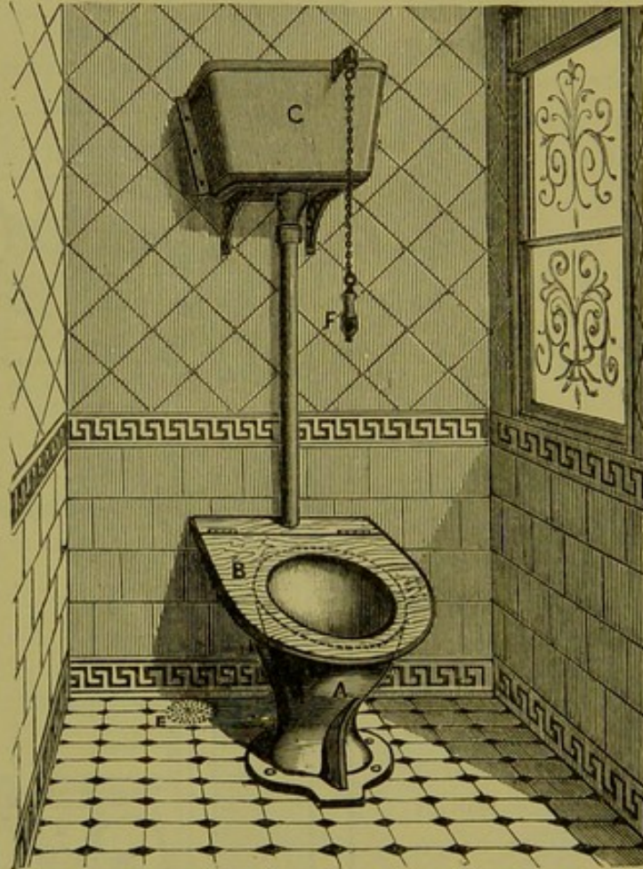
FIG. 186.—View of the Pedestal "Hygienic" [o] Wash-down Closet with "Flat-back" Syphon Flushing Cistern, c.
