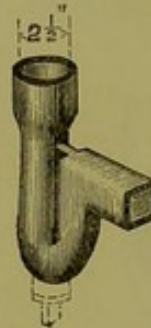
FIG. 30.—View of 1\frac{1}{4} -in. "Anti-D-trap," with enlarged mouth.
