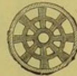
FIG. 259.—Sunk plug "Washer" and "Cobweb" Grating.
