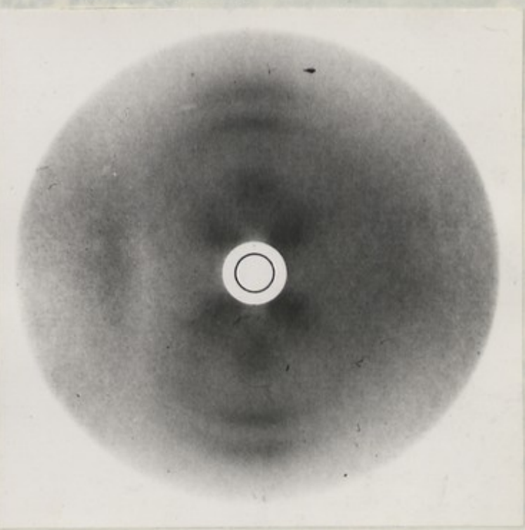
PLATE 2 Sheet specimen of herring sperm NaDNA. X-rays in plane of sheet. 90% Relative Humidity. Exposure 5 hours N.B. In each case direction of shear in sheet is meridional. multi-fibre specimen technique.
