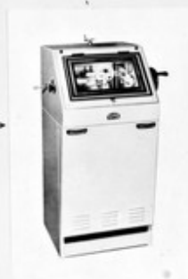
SECTIONS CUT ON A CRYOSTAT (refrigerated microtome) OPERATED IN A DARKROOM UNDER A SAFELIGHT
