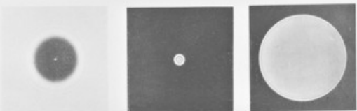
(a) Point source and circular obstacle. (b) Point source and small circular aperture. (c) Point source and large circular aperture.
