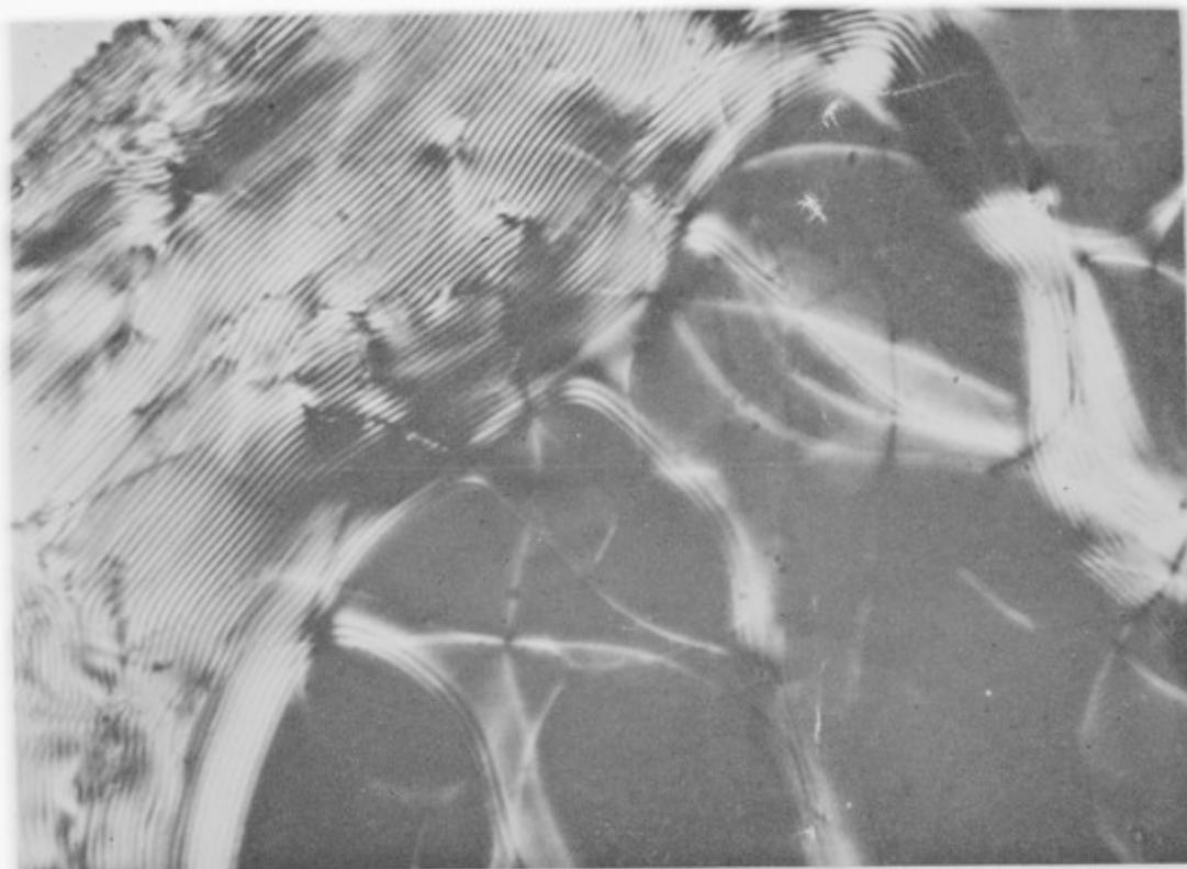
Fig. 8. Uniform areas with surrounding system of periodic lines. Solution of PBLG in dioxane in circular cell, 1 mm deep. The line system is largely concentric with the circumference of the cell, a small arc of which can be seen in the top left-hand corner. S = 21 \mu . Polars at 45^\circ . The uniform areas appeared bright blue.
