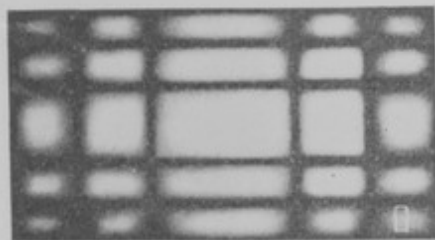
FIG. 94.—Pattern due to rectangular aperture; point source of light (Lummer und Reiche).
