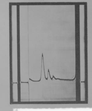
Multiple schlieren peaks show presence of several sedimenting components
