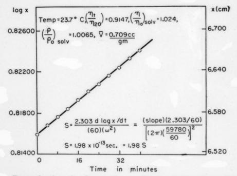
Determination of sedimentation coefficient of ribonuclease from a plot of log x (x is the distance of boundary to axis of rotation) versus t (t is the time in minutes).
