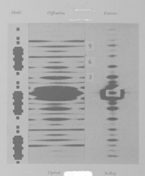
Comparison of the model for the moist fibril with corresponding optical and X-ray diffraction. Here, background covers 0.54 of the macroperiod, with centre at 0.18 relative to d and horizontal width 2.5 times that added by bands.
