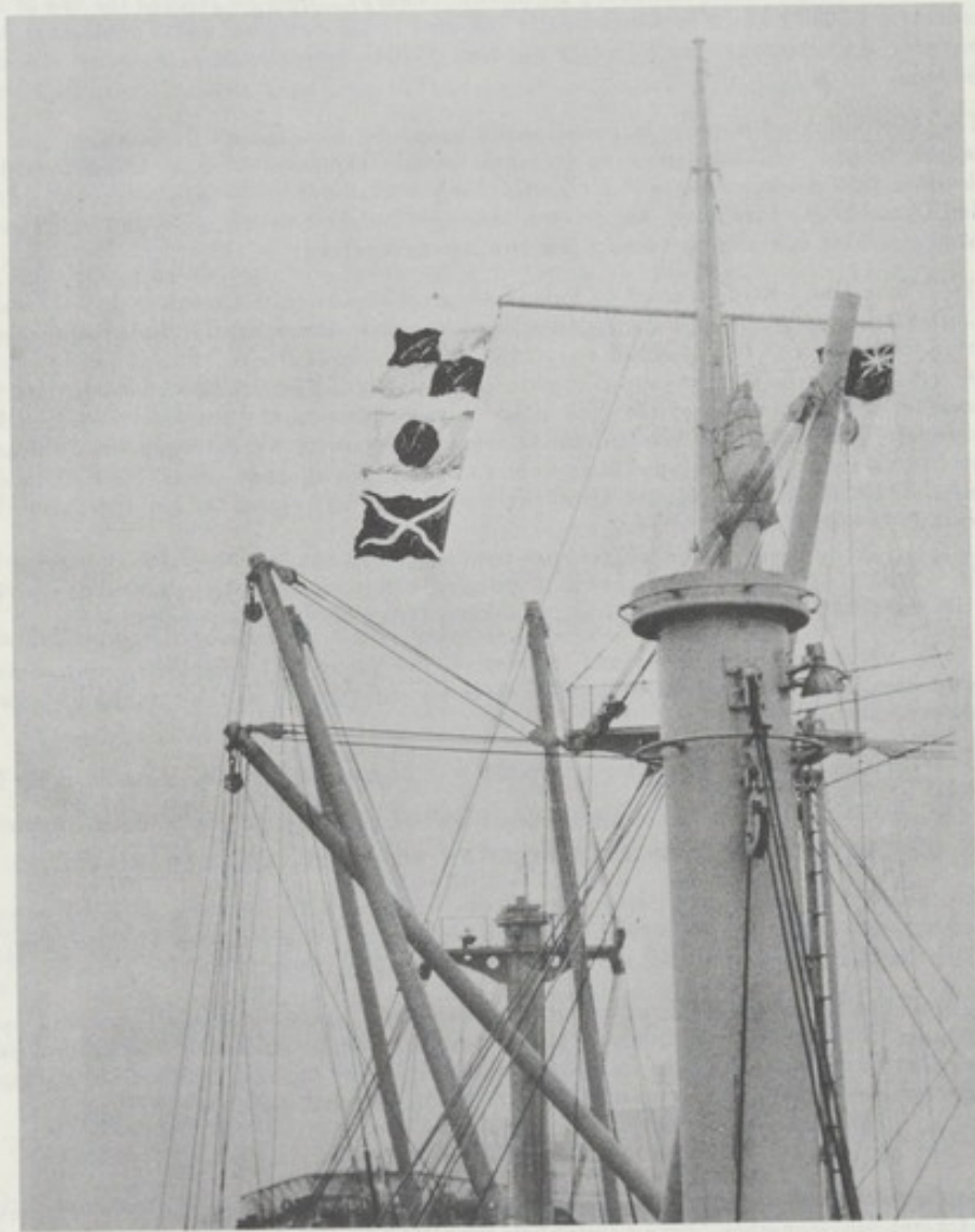
"I require Port Medical Officer" - The Flag Signal "L.I.M." on an incoming ship
