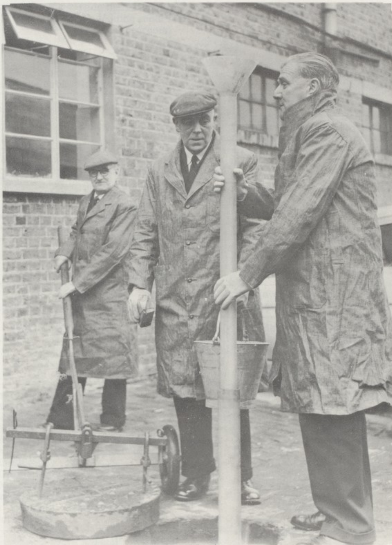
RODENT CONTROL IN SEWERS telescopic device for laying baits in deep manholes.
